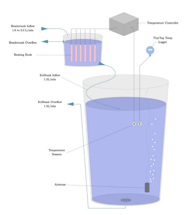
Schematic overview of experimental tank holding 200 individual krill. Light conditions were kept constant, temperature was regulated within a range of 0.1°C. Krill were fed ad libitum.
