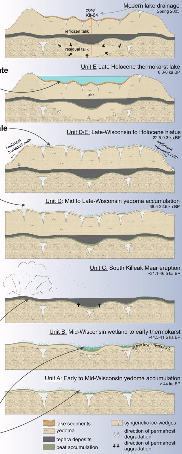
lake sediments, yedoma, tephra deposits, peat accumulation, syngenetic ice-wedges, direction of permafrost degradation, direction of permafrost aggradation
