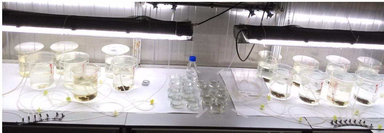
Figure 12. Bigger plastic beakers of the competition experiment between A. esculenta and L. digitata at 5 and 15°C. Compressed air ventilation was established to build up a proper environment for the growing sporophytes.
