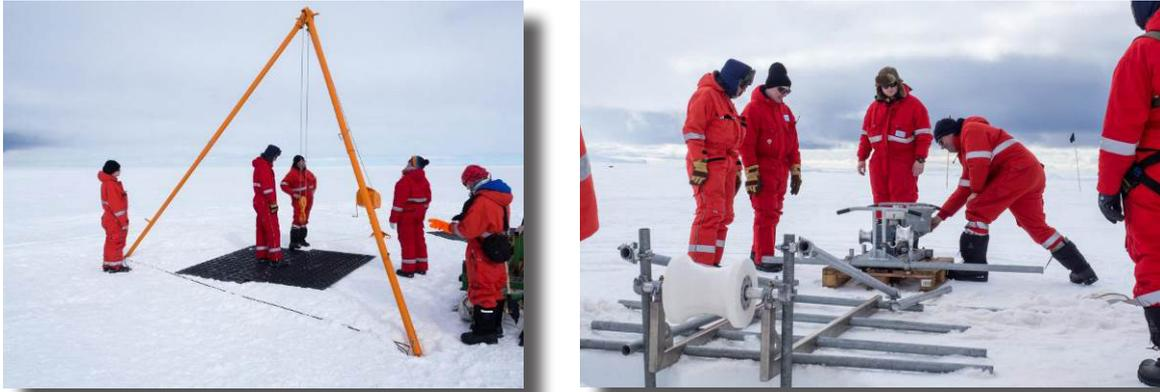
*Fig. 3.1.1.9: Left: The tripod (test set-up, ultimately to be placed over the hole for lifting heavy instruments). The area covered by black plates (2 x 2 m) indicating the approximate size of the hole. Right: The rope-guidance at the edge of the hole for the recovery of the mooring rope. Pulling out the rope is supported by the portable capstan (behind the rope-guidance).*
