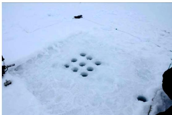
*Fig.3.3.1.13: Image of a typical coring grid taken at the L-arm site. The core hole on the right side was used to deploy the sensors attached to a L-arm underneath the ice. The ice cores were taken at the centre of the square in which the light measurements are performed. Picture by André Maijboom (IMARES).*
