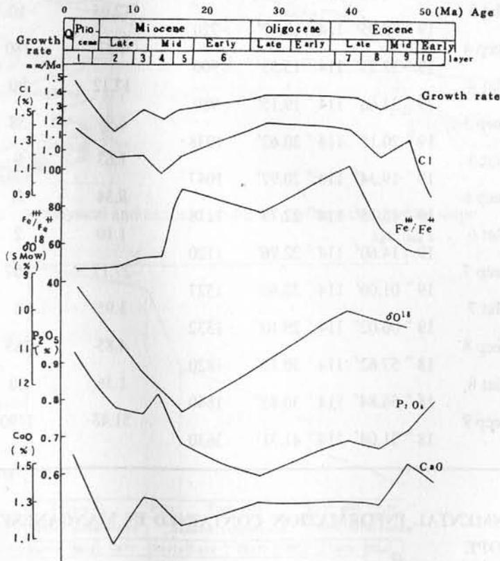
Fig.3 Variation of growth rate, chlorine,  $\text{Fe}^{3+} / \text{Fe}^{2+}$ ,  $\delta\text{O}^{18}$ ,  $\text{P}_2\text{O}_5$  and CaO content in manganese crust.
