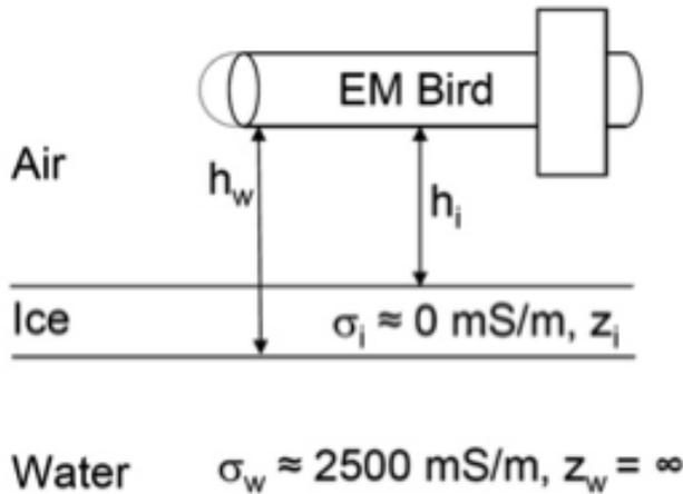
**Figure 4.13:** The EM-Bird system measures the distance  $h_w$  above the ice-water interface as the field strength of a secondary EM field and the distance  $h_i$  above the ice with a laser altimeter. Difference of distances gives the ice thickness  $z_i$ . Here,  $\sigma$  denotes the conductivity of the media. From [Haas et al., 2009]
