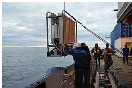
Fig. 3: The Ultra-Clean Rosette on its way to the water. Photo: Micha Rijkenberg
