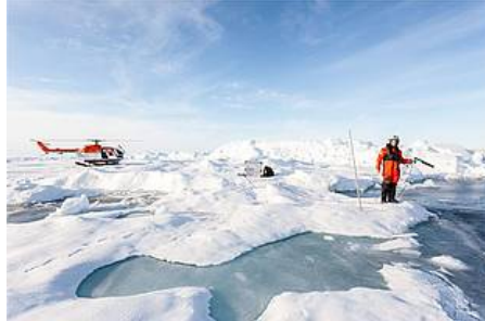
Fig. 4: Mario Hoppmann on an ice flow. He measures a temperature and salinity profile with an XCTD. Foto: Sergey Pisarev
