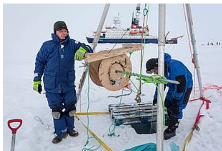
Fig. 4: Sergey and Nicolas prepare the lowering of an 800 m long cable for an atmosphere-ice-ocean-observing system. Photo: Mario Hoppmann (Photo: Alfred Wegener Institut)
