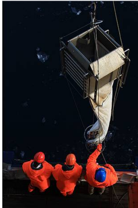
Fig. 1: The multi net is lowered to the water. Photo: Imke Petersen (Photo: Alfred Wegener Institut)
