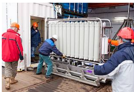
Fig. 2: The Ultra-Clean-Rosette leaves the Ultra-Clean Container for the next cast. Photo: Mario Hoppmann (Photo: Alfred Wegener Institut)
