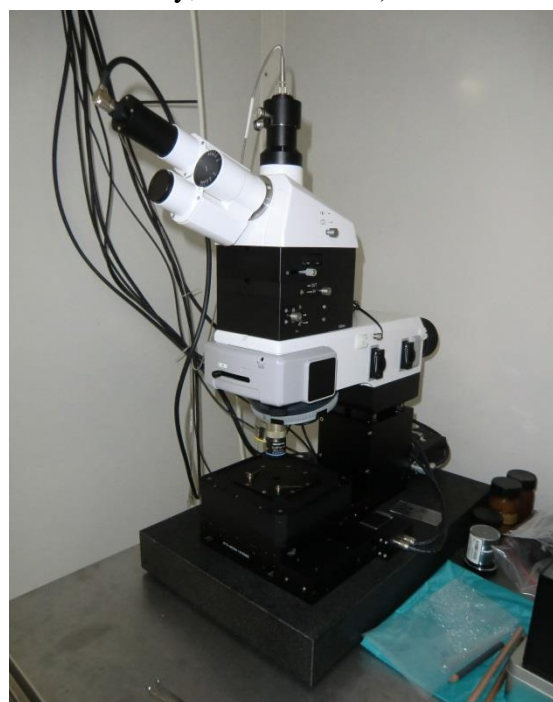
Fig. 16: The Raman microscope in the cold laboratory of the Alfred-Wegener-Institute
