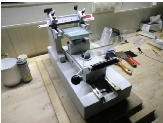
Fig. 10: A microtome used for the preparation of thin sections (KLEITZ 2013)
