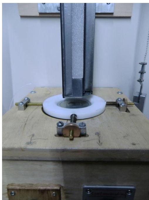
Fig. 13: A firn core before the melting process starts (CFA system of the Alfred-Wegener-Institute for Polar and Marine Research) (KLEITZ 2013)
