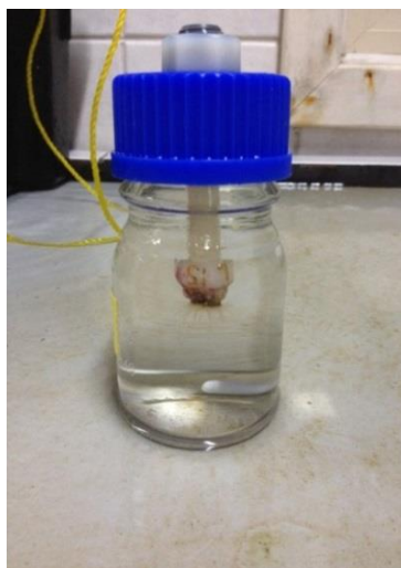
Figure 13: Coral glued on a screw, screwed-in the lid of a 100ml Schott bottle.
