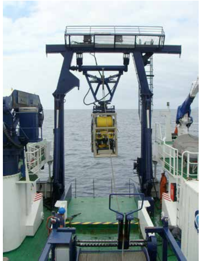
Figure 1: Liropus 2000 ROV deployment using the A-frame in the stern deck of R/V Ángeles Alvariño during the MIDAS-EL HIERRO cruise. ROV is located inside the TMS (framework in the middle of the image with the yellow umbilical on top).
