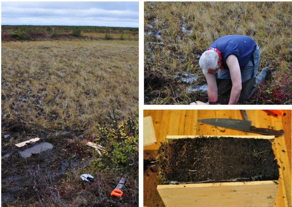
Fig. 6-3: Collection of the peat profiles: Left: Location AE-7 after removal of the profile, right top: manual removal of the cut-free profile AE-7; right bottom: storing the adjusted profile AX-29 in a wooden box.
