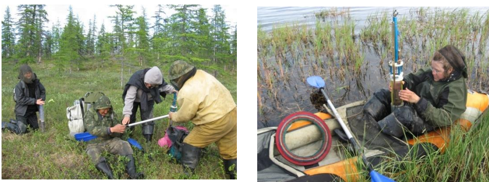
Figure 13: Preparation and securing of the short core with the UWITEC gravity corer (Photos: U.Herzschuh, S.Müller, 2007).
