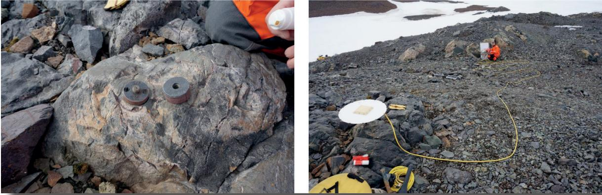
*Fig. 4.4.3: Installation of the GPS equipment at the sites PRA1. The left photograph shows the existing GAP (Geodetic Antarctic Project) marker from 1995. The right photo shows the mounted GPS antenna in the left foreground.*
