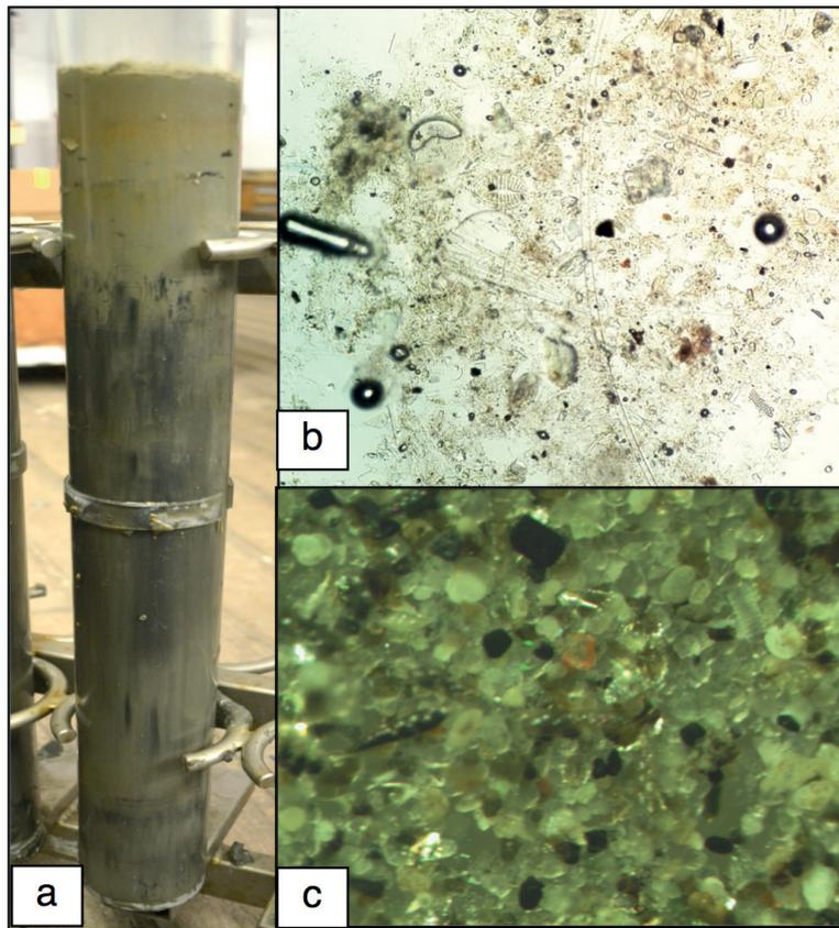
*Fig. 3.2.3: MUC tube retrieved at station PS97/054-2 (a; J. Müller). Microscope images of the fine fraction from the surface layer (b; L. Rebolledo) and of the coarse fraction from the base of the MUC (c; H. Schulz) permit an immediate micropaleontological and sedimentological characterization.*
