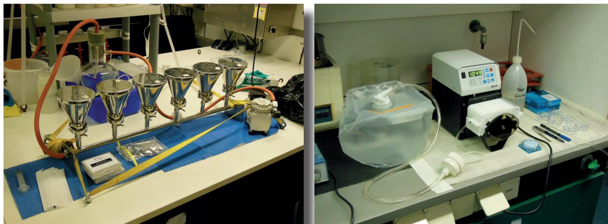
Fig. 8.2: Filtration plant set-up for water samples to determine chlorophyll a and silicate in shipboard wet chemistry laboratory, filtration device for coccolithophore filtrations samples in the background (left). Peristaltic pump set up for suspension filtration of IOW water samples (right).
