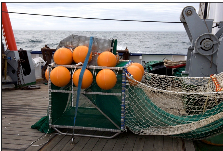
Figure 2: Fish-lift attached to the juvenile fish trawl of RV Heincke (photography: F. Mark).
