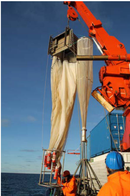
Fig. 7.2: Multinet Type Maxi with additional net bag for non-quantitative, depth-integrated zooplankton sampling.
