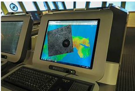
Fig. 4: IceGIS on Polarstern's bridge. The bridge radar is shown, projected on the latest satellite image of the sea ice cover and bathymetry in the background. (Photo: Alfred-Wegener-Institut / T. Krumpfen)
