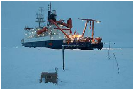
Fig. 3: Buoy station on sea ice. The station consists of a sea ice mass balance buoy, measuring sea ice thickness and solar radiation above and under the sea ice, and a snow buoy, measuring snow depth and air temperature. (Photo: Alfred-Wegener-Institut / M. Nicolaus)
