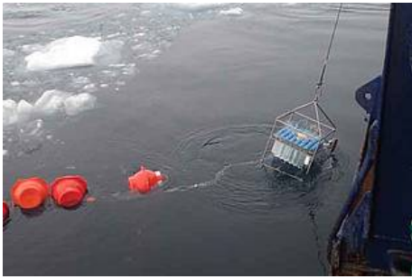
Fig. 8: RAS 500 Water sampler during recovery of the central Arctic Ocean mooring (Photo: AWI / A. Purser)
