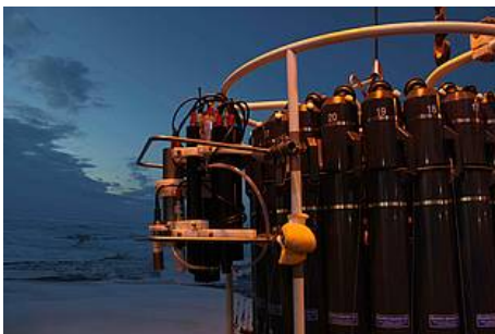
Fig. 5: To obtain a continuous Nitrate and pCO 2 profile from the surface down to 500m water depth a set of Nitrate and pCO 2 sensors are attached to the CTD rosette. (Photo: AWI / D. Scholz)
