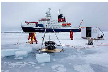
Fig. 2: Installation of a sea ice station using with the "Beast" for under-ice measurements. The ROV is deployed through the hole in the ice and is operated from the control stand, which is mounted on two sleds. (Photo: Alfred-Wegener-Institut / M. Schiller)
