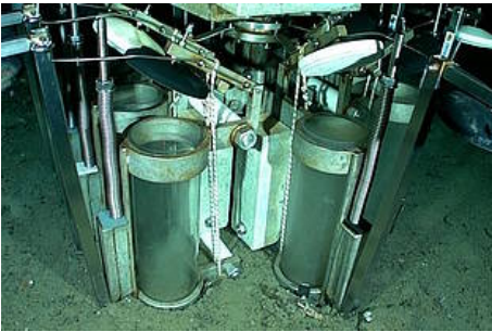
Fig. 8: A sample is taken with the TV-guided multiple corer. (Photo: TV-MUC, AWI)
