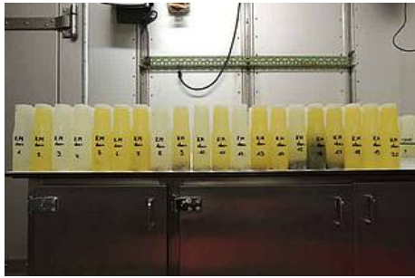
Fig. 9: Sediment trap bottles from a multisensory mooring, which collected sinking particles year round in the Central Arctic Ocean. (Photo: Alfred-Wegener-Institut / D. Scholz)
