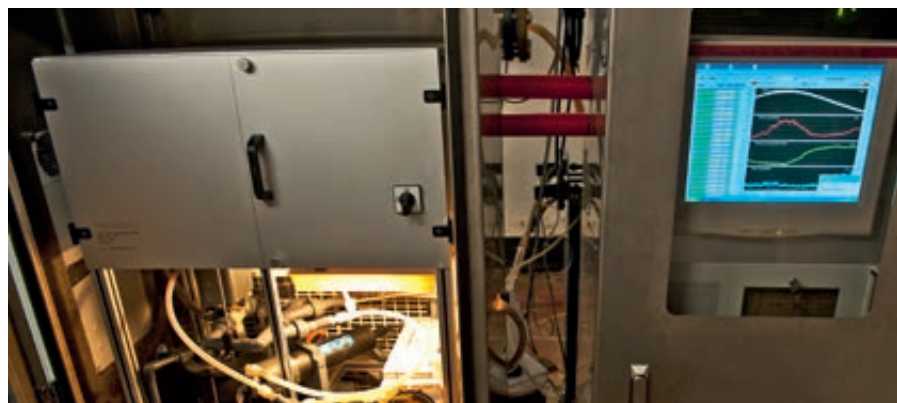
Packed full with measuring devices and sensors, the FerryBox provides live data on condition of the sea via a direct line to the researchers. Photo: U. Nettelmann
