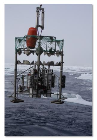
Fig. 9.1: Benthic Lander System with transecting microprofiler and 3 benthic chambers
