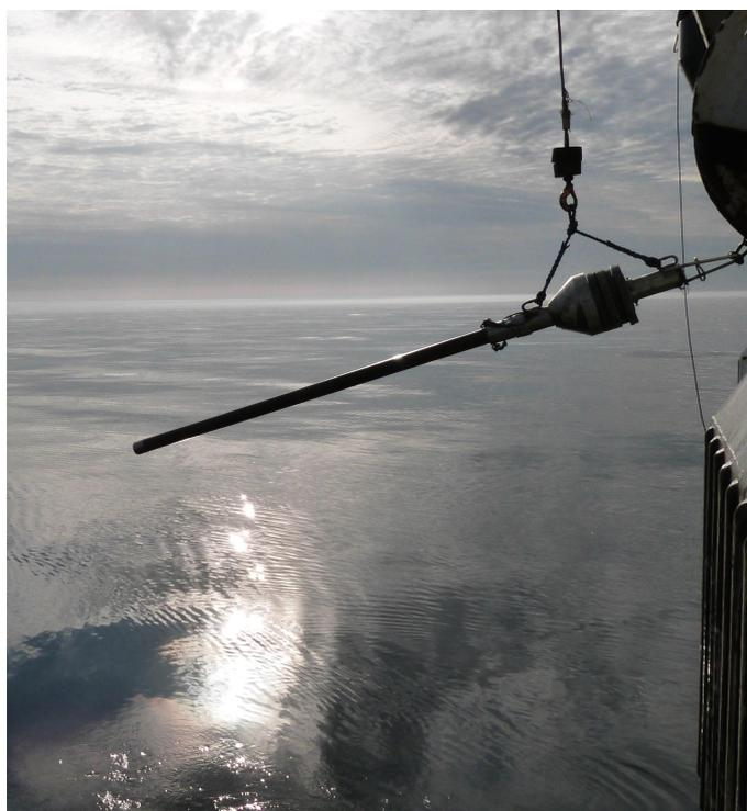
*Figure 5: A gravity core is retrieved and brought on board in near horizontal position.*
