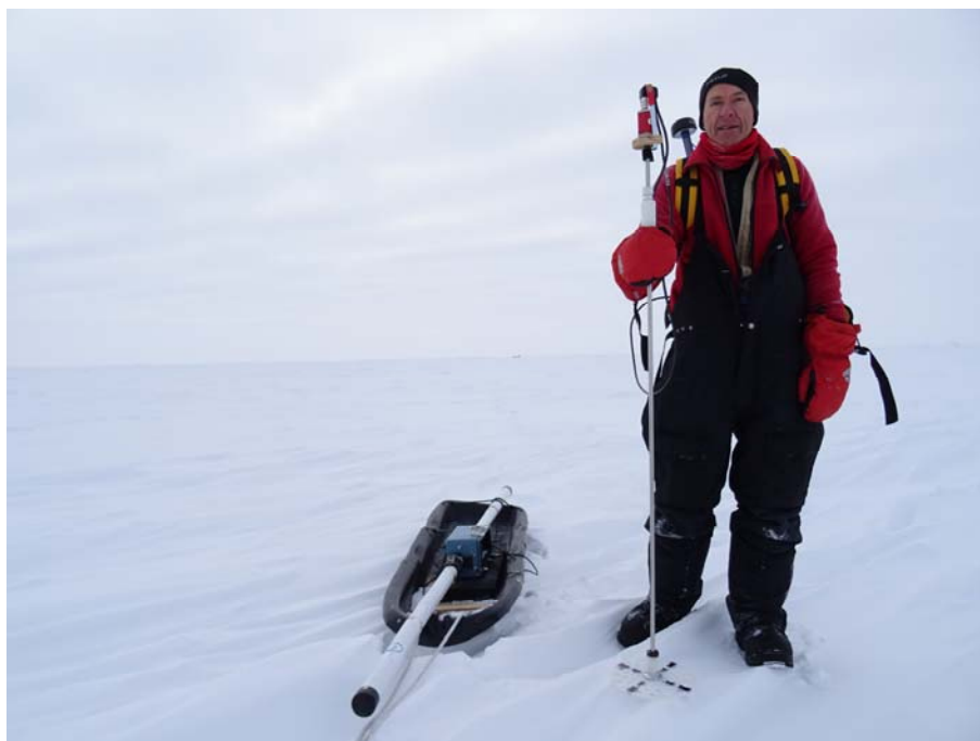
Figure S1. Photo of the EM31SH ice thickness sounder and Magnaprobe snow thickness sensor used in this study. The EM instrument is strapped onto a toboggan dragged by one person and operated in horizontal dipole mode. The Magnaprobe is carried by another person. Note rather level ice surface morphology (Site 5; cf. Figure 2) and Twin Otter aircraft in the background (small black spot).
