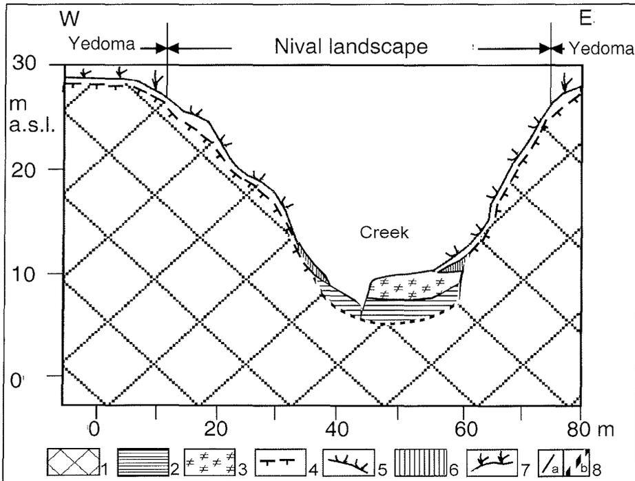
**Fig. 7:** Schematic profile of the „cold“ snow patch No. 1 (ravine type) and the surrounding nival landscape at Bykovsky Peninsula. 1: Ice Complex; 2: stratified ice; 3: stratified firm; 4: boundary of the active layer; 5: silt with plant detritus from the surface of the active layer; 6: talus; 7: surface of the active layer with plant cover of Subarctic grass tundra; 8: lithologic boundaries: 8a: determined, 8b: supposed.
