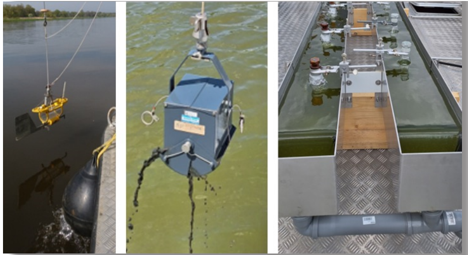
Fig. 4.2: Horizontal water sampler and sediment sampling at Albis (Photos by N. Kamjunke)
