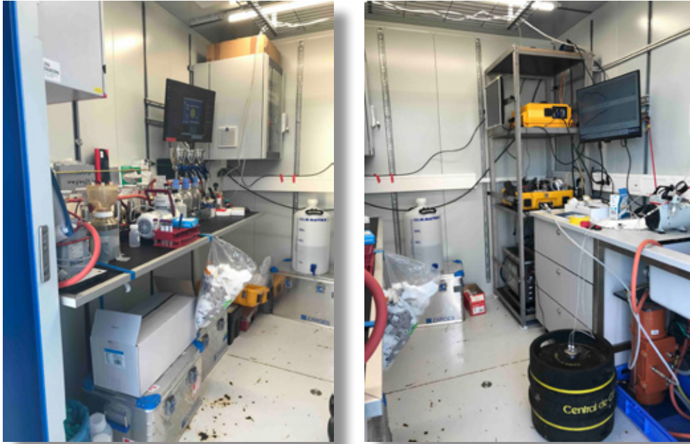
Fig. 6.2: Instrument set-up in the MOSES lab-container, with FerryBox and LosGatos on the right side and water sampling set-up on the left side. (Photos by I. Bussmann)
