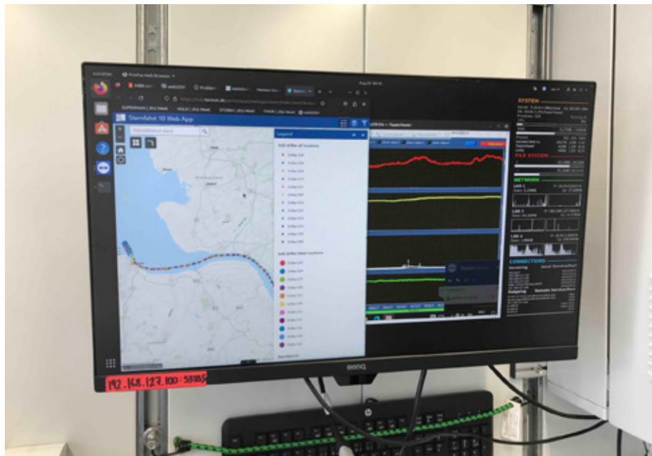
Fig. 6.19: Screen in the lab-container displaying the position of the transponders and the basic hydrographic parameters from the FerryBox. (Photo by I. Bussmann)
