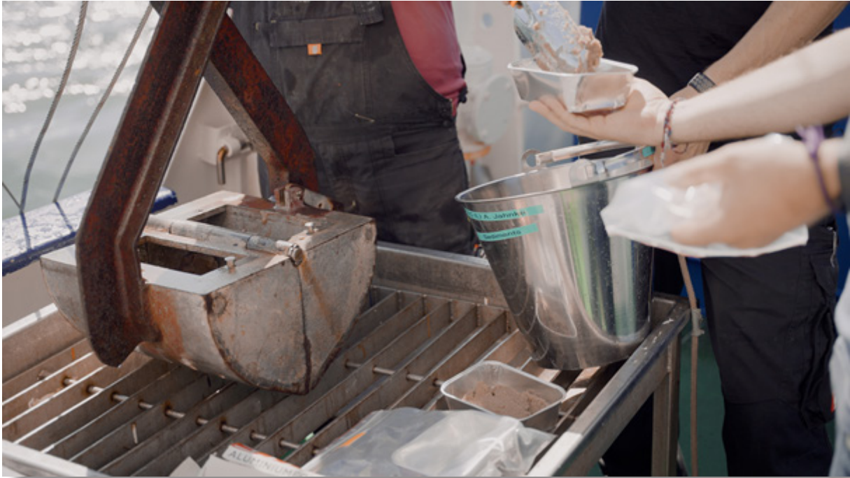
Fig. 6.14: Processing sediment samples from a Van-Veen grab. (Photo by I. Reinisch)
