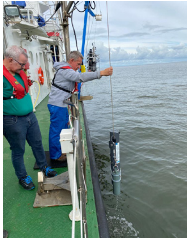
Fig. 6.5: Sampling with the 'Goflo' multi-element sampler (Photo by H. Brix)
