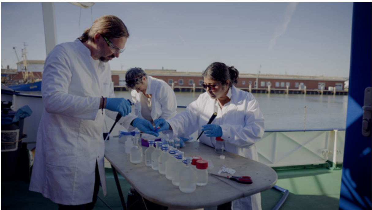
Fig. 6.15: C. Faber and S. Bhattacharya poisoning DIC samples on deck in the harbor of Büsum. (Photo by I. Reinisch)
